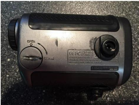
**BUSHNELL TOUR V2 SHOWING PLACEMENT OF THE BELT CLIP TAB/3M ADHESIVE DISK ASSEMBLY ON THE LASER LENS END OF THE V2**
